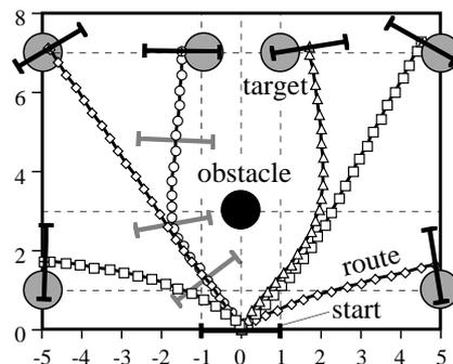
Figure 8: Comparison of the robot’s routes after learning between in the task with an obstacle and with no obstacles.
