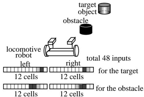
Figure 7: Simulation environment of “going to a target” task with an obstacle
